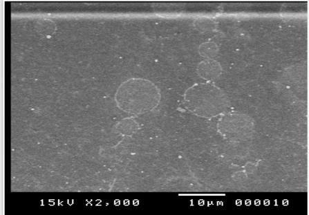
Two IOLs, one showed wrinkled optical surface the other IOL showed some deposits over the optical surface of the lens, both were of the hydrophobic type
