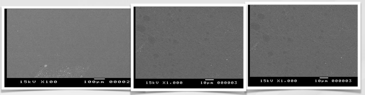
Two IOLs shows no identifiable marks with clean polished optical surface
